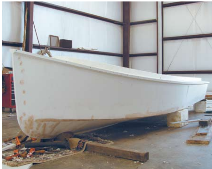
Once glued and finished, seams in a PVC skiff are difficult to see. Screws are used to pull the edges tight but could be removed once the glue sets up, Andy Cockrell says.
